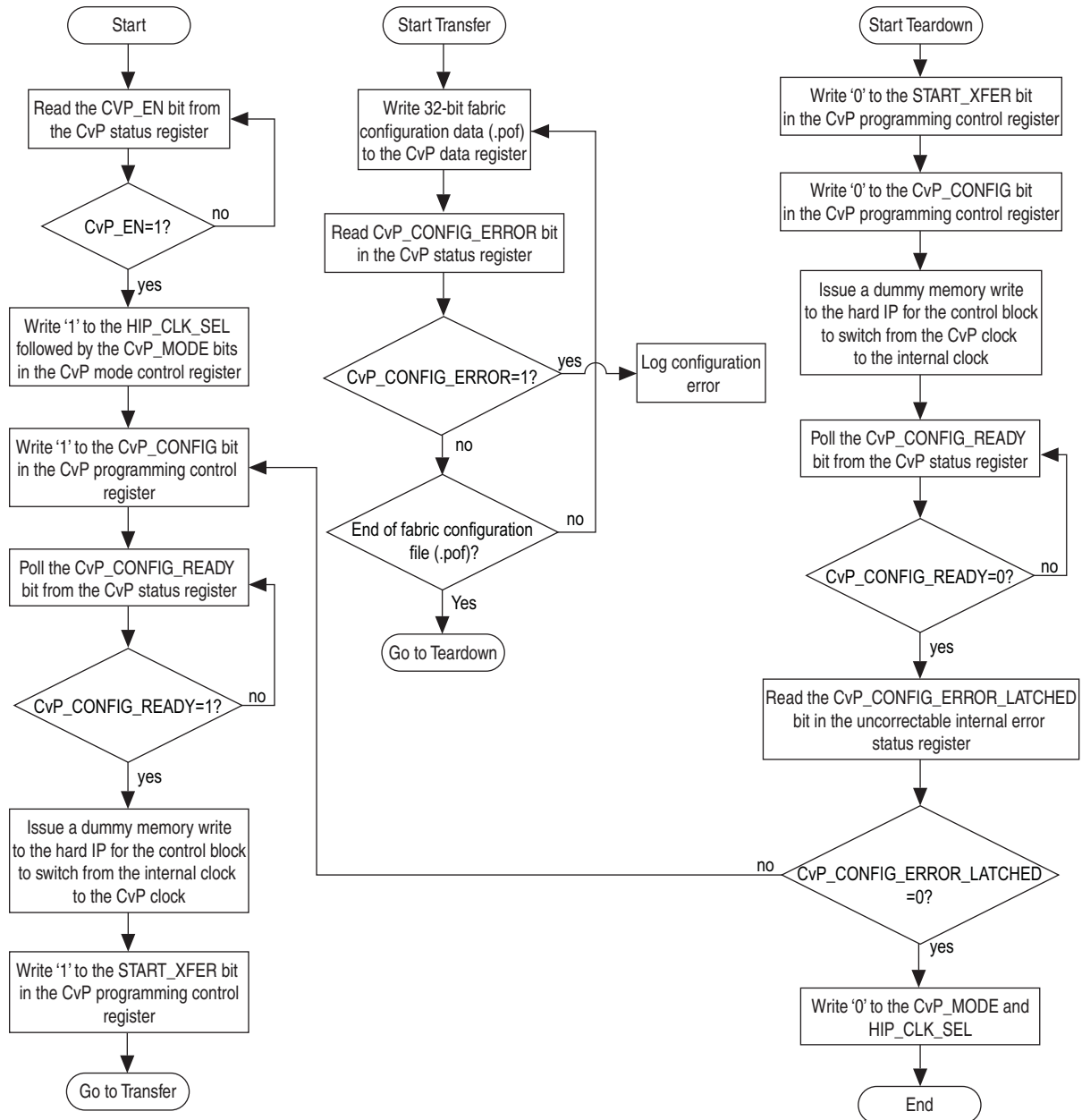
Figure 6-1. PCIe Driver in the PCIe Host Configuring the FPGA Fabric via PCIe Link
