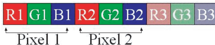
Figure 4. Subpixel Organization on a Standard LCD
