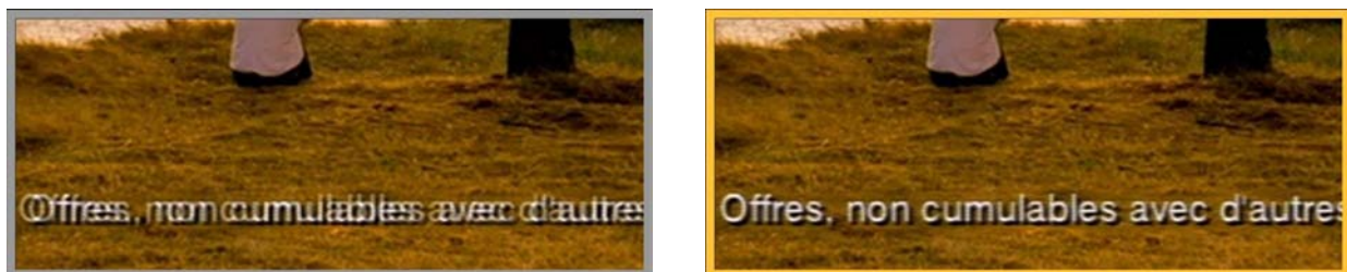
Figure 2. Visual Quality of Moving Text Produced by Traditional Upscaling Algorithms (left) vs. Advanced Upscaling Algorithms (right)
