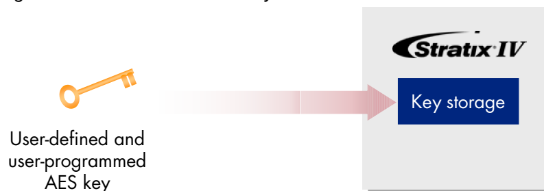
Figure 1. Step1: Program Stratix IV Device With Key
