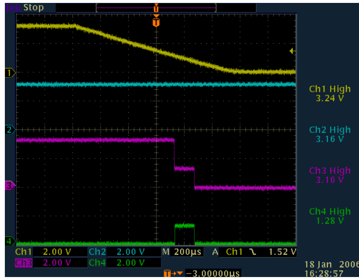
Figure 8. V_{CCINT} Ramps Down, V_{CCIO} Is Steady at 3.3 V, Output Pins With External 10-k \Omega Pull-Down Resistor
