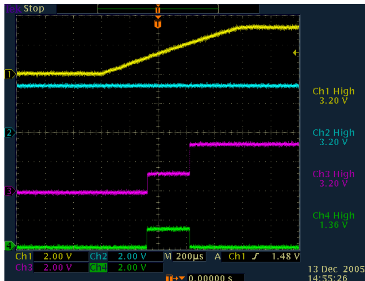
Figure 5. V_{CCINT} Ramps Up, V_{CCIO} Is Steady at 3.3 V, Output Pins With External 10-k \Omega Pull-Down Resistor
