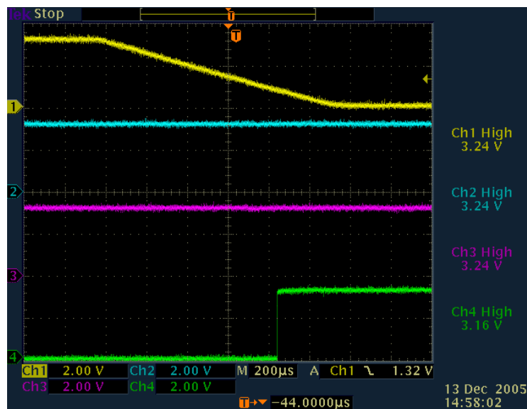
Figure 7. V_{CCINT} Ramps Down, V_{CCIO} Is Steady at 3.3 V, Output Pins With External 10-k \Omega Pull-Up Resistor
