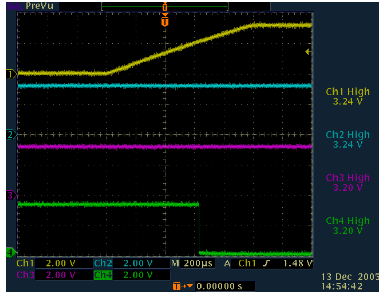
Figure 4. V_{CCINT} Ramps Up, V_{CCIO} Is Steady at 3.3 V, Output Pins With External 10-k \Omega Pull-Up Resistor
